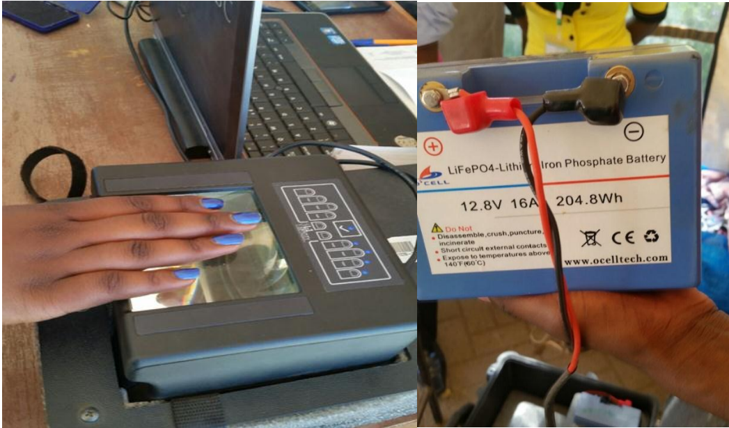
Figure 1: The photo collage above shows: The BVR kit (finger print scanner, laptop and camera) at one of the VR centers in Kajiado north constituency – Kenya and the battery back-up in the event of power cuts. Each of the centers that we visited had 2 reachable batteries that could last for at least eight hours each.
